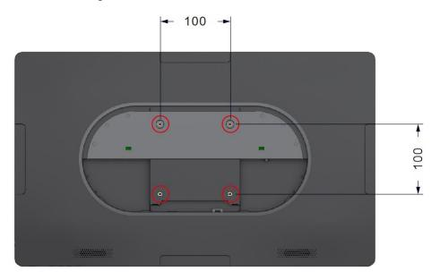
The monitor may be mounted horizontally (output connectors facing down) or vertically (output connectors facing right). Ensure that the surface material and the standard VESA wall mount bracket (purchased separately) are strong enough to support the weight of the monitor (refer to the Specifications table below for weight information).
