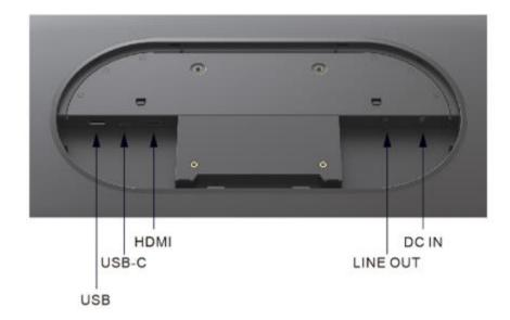
DC IN: Optional power connector (Center pin: + 12 vdc; Barrel: ground).
