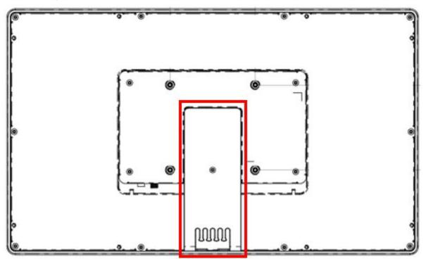
A cable management bracket, outlined in red below, is attached to the back of the monitor:
