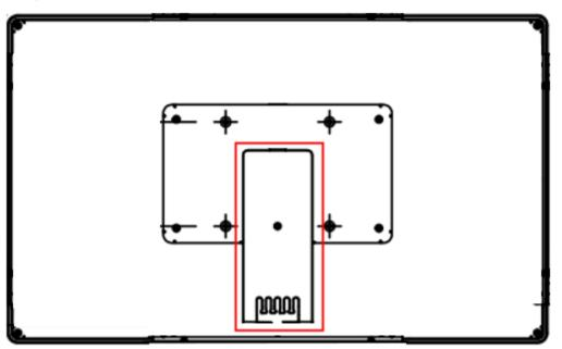
A cable management bracket, outlined in red below, is attached to the back of the monitor:
