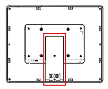
It has five cable slots and a central opening below, centered. The bracket, attached by a single screw, can be removed if desired to facilitate cable connections, then reattached. The slots can hold smaller diameter cables; larger diameter cables can be nested within the confinement area.
