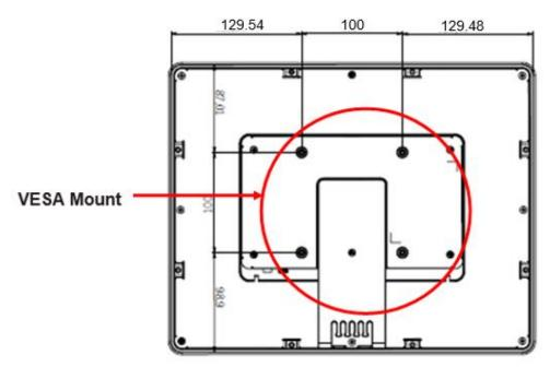
The monitor has an integral VESA standard mount pattern that conforms to the "VESA Flat Display Mounting Interface Standard" which defines a physical mounting interface and corresponds to the standards for monitor mounting devices.
